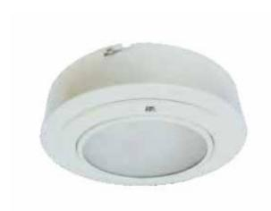
Decorative surface mounting integral LED downlight luminaire comprising of sheet aluminium housing in white powder coated finish with PMMA diffuser & inbuilt constant current electronic driver
