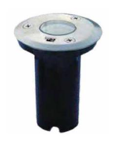
Decorative around / wall recess mounting Integral drive over/walk over HP LED ground burial luminaire comprising of die cast aluminium housing with cover ring in stainless steel finish & toughened/frosted glass, with inbuilt constant current electronic driver.
