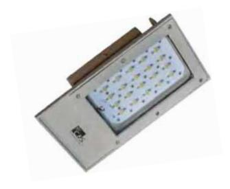
Decorative HP LED street light luminaire with 120 degree X 60 degree streetlight photometry with lens optics on LEDs, comprising of single piece pressure die cast aluminium alloy LM24 housing with heat resistant toughened printed glass & constant current inbuilt electronic driver.
