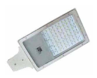
Decorative HP LED street light luminaire with wide photometry, comprising of single piece pressure die cast aluminium alloy LM24 housing with heat resistant toughened printed glass & constant current inbuilt electronic driver
