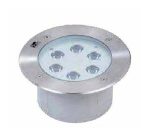
Decorative around/wall recess mounting Integral drive over/walk over HP LED ground burial luminaire comprising of die cast aluminium housing with cover ring in stainless steel finish & toughened/frosted glass, with inbuilt constant current electronic driver.
