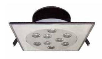
Decorative recess mounting LED downlight luminaire comprising of brushed stainless steel finish housing with transparent lens & external constant current electronic driver
