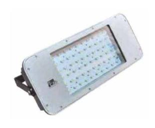
Decorative HP LED flood light luminaire with 60 degree X 60 degree floodlight photometry comprising of single piece pressure die cast aluminium alloy LM24 housing with heat resistant toughened printed glass & constant current inbuilt electronic driver.
