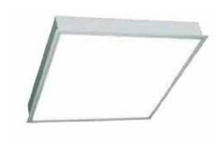
Decorative recess mounting integral LED modular ceiling luminaire comprising of powder coated sheet steel housing with extruded aluminium powder coated frame with diffused PMMA refractor & internal constant current electronic driver.
