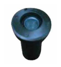
Decorative recess mounting Integral drive over/walk over HP LED ground burial luminaire comprising of die cast aluminium housing with cover ring in stainless steel finish & toughened/frosted glass, with inbuilt constant current electronic driver.
