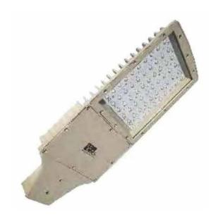
Decorative HP LED street light luminaire with 120 degree X 60 degree streetlight photometry with lens optics on LEDs, comprising of single piece pressure die cast aluminium alloy LM24 housing with heat resistant toughened printed glass & constant current inbuilt electronic driver.
