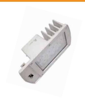
Decorative HP LED street light luminaire with wide photometry, comprising of single piece pressure die cast aluminium alloy LM24 housing with heat resistant toughened glass & constant current inbuilt electronic driver.
